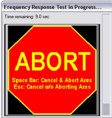
**Note:** If your axis faults during the test, it is most likely due to Position Error Limit. By default, the limit value is set to 1000. You will need to increase this to a reasonable number due to the high resolution of the S200 drive.
